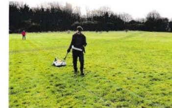
Above: GPR survey on Quoy Meadow with 50 MHz antenna
