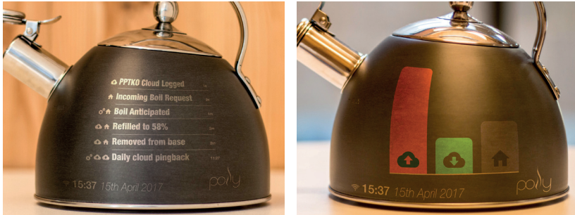
Figure 8. Left: In order to underscore trust in the device, Polly's timeline shows every data transaction the kettle takes place in. Right: The data volume graph helps the user to understand how much data the kettle is uploading or downloading by showing relative volumes next to each other visually.
