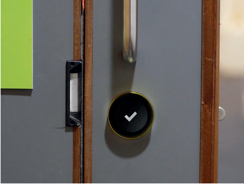
Figure 18. Image of the IoT lock mounted on a door
