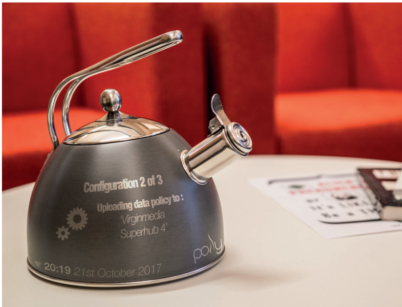
Figure 9. Using a fictional standard called Minimum Necessary Datagram Protocol, Polly creates a machine-readable file that integrates with compatible routers. This acts as a self-imposed firewall, and ensures the kettle can send or receive only data that the user has specially agreed to.
